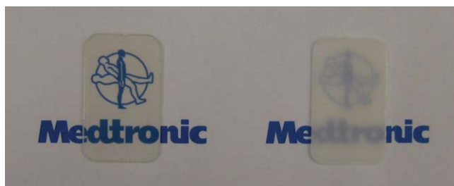
Figure 5 A piece of PLGA/PTMC (80/20 wt) film (about 1 mm thick) was placed over a word “Medtronic” (left). The word is legible. A piece of PLGA/PCL film with similar thickness was placed over a same word. The word is illegible (right). This indicates the PLGA/PTMC film is more transparent than the PLGA/PCL film. [Color figure can be viewed in the online issue, which is available at www.interscience.wiley.com .]
